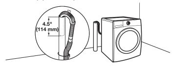
Minimum diameter for a standpipe drain: 2" (51 mm). Minimum carry-away capacity: 17 gal. (64 L) per minute. A 1/4" (6 mm) diameter to 1" (25 mm) diameter Standpipe Adapter Kit is available (Part Number 3363920). Top of standpipe must be at least 30" (762 mm) high; install no higher than 96" (2.44 m) from bottom of washer. If you have an overhead sewer and need to pump higher than 96" (2.44 m), a sump pump and associated hardware are needed. See "Alternate Parts".
