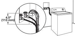
See requirements for floor standpipe drain system.
