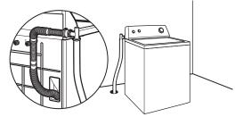
Floor drain system requires a Siphon Break Kit and additional drain hose that may be purchased separately. See "Tools and Parts". Minimum siphon break: 28" (711 mm) from bottom of washer. (Additional hoses might be needed.)
