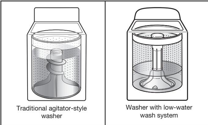
The washer automatically adjusts the water level to the load size—no water level selector is needed.
