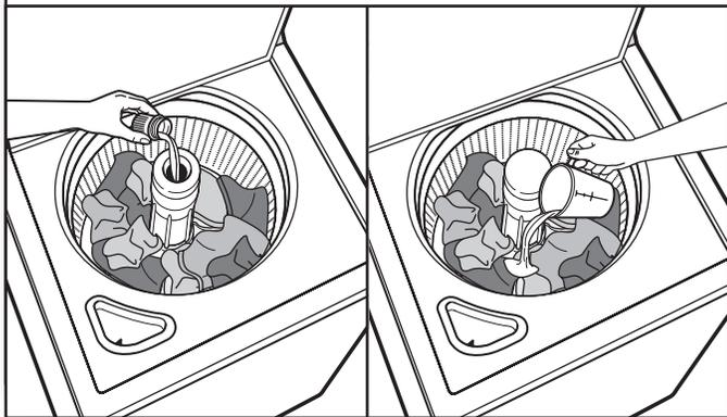
During the final rinse, wait until the washer has completed filling, press the START/Pause button to pause the washer. Lift the lid and add the measured recommended amount of liquid fabric softener. Do not use more than the recommended amount. Close the lid and press the START/Pause button again to start the washer.
