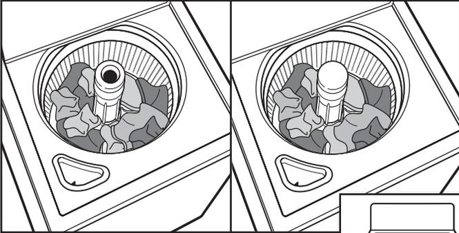
Load garments in loose heaps evenly around basket wall. For best results, do not pack the load tightly. Do not wrap large items such as sheets around the agitator; load them in loose piles around the sides of the basket. Try mixing different sized items to reduce tangling.
