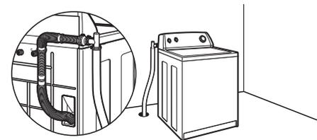
Minimum diameter for a wall or floor standpipe drain: 2" (51 mm). Minimum carry-away capacity: 17 gal (64L) per minute. Top of standpipe must be at least 39" (991 mm) high; install no higher than 96" (2.4 m) from bottom of washer. A sump pump system is required for higher installations.
