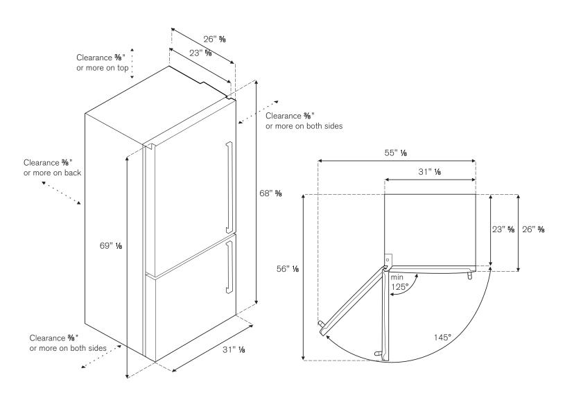
INSTALLATION: There shall be a space not less than 3/8 inch from the top of your refrigerator, not less than 3/8 inch from both sides and 3/8 inch or more from the back of the refrigerartor to the adjacent walls respectively. This requirement is necessary to create clearance in order to open and close the door as well as to avoid the spacing for adequate ventilation around the refrigerator.
