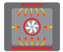
Bertazzoni dual-fuel ranges are equipped with extra-wide European convection ovens with heat-assisted convection fan, providing balanced air flow and even heat distribution.
