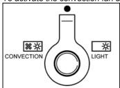
Turn the knob anti clockwise for activation of the convection fan +light Turn the knob clockwise to turn on the oven light.
