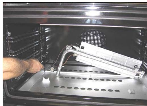
Unscrew the nozzle located inside the gas fitting using a 10 mm [ socket wrench].
