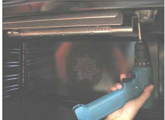
Using a 7 mm [name of the tool] unscrew the nozzle. Replace the nozzle using the conversion set supplied with the range or by a Bertazzoni authorized parts warehouse. Each nozzle has a number indicating its flow diameter printed on the body. Consult the table on page 20 for matching nozzles to burners.
