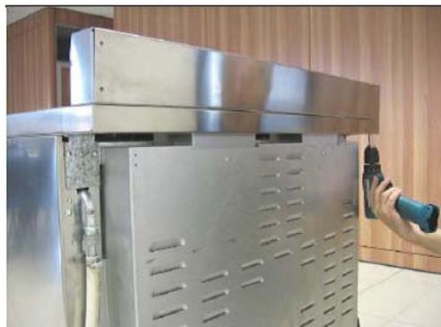
Connect the back and front part of the upstand. Check for tight assembly.
