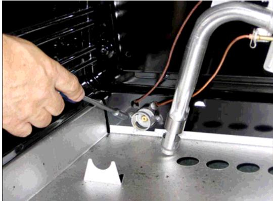
Adjust the primary airflow by loosening the screw P and setting the gap X in the Venturi cone to 1/2" (5/16" for natural gas).
