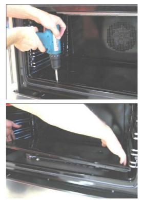
Loosen the screw located on the right side of the burner and pull out the burner from its support.
