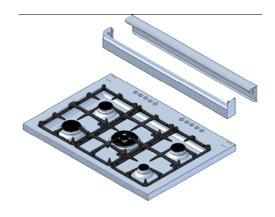
Disassemble the backguard and position the front part on the worktop. Align the screw holes with the corresponding holes at the back of the worktop.
