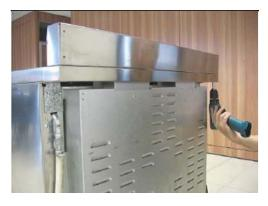
Connect the back and front part of the upstand. Check for tight assembly.
