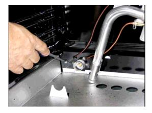
Adjust the primary airflow by loosening the screw P and setting the gap X in the Venturi cone to  $\frac{1}{2}$ " (5/16" for natural gas).
