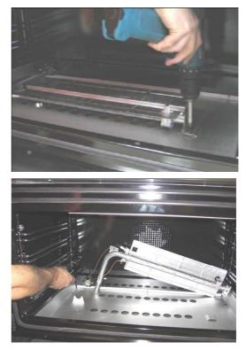
Unscrew the nozzle located inside the gas fitting using a 10 mm [ socket wrench].
