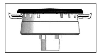
3. Always adjust the burner flame so it does not extend beyond the edge of the pan.
