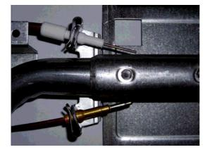
The tip of the spark plug or thermocouple must fully overlap at least the first gas emission hole of the burner.
