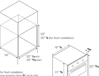
\* for flush installation leave monting strips %" each side
