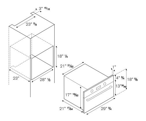
The minimum gap between the kichen cabinet upper or lower panel and the appliance is 1/8. This dimension must be added to the height listed in the drawings
