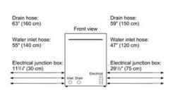
All connections are at the rear of the appliance. Extension for drain hose available as accessory. Power cord for connection to electrical outlet (3-prong plug) available as accessory.
