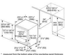
measured from the bottom edge of the countertop panel thickness recommended <sup>3</sup>/4" (20 mm), panel weight 7-22 lbs (3-10 kg)
