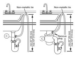
Note: Plumbing installations will vary - refer to local codes. Drain hose included is 79 (201 cm) and can be extended to a maximum of 155 3/4" (396 cm).
