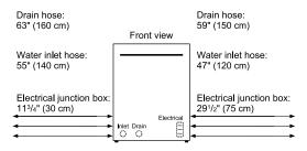
All connections are at the rear of the appliance. Extension for drain hose available as accessory Power cord for connection to electrical outlet (3-prong plug) available as accessory.
