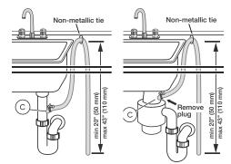
Note: Plumbing installations will vary - refer to local codes. Drain hose included is 79 (201 cm) and can be extended to a maximum of 155 3/4" (396 cm).
