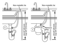
Note: Plumbing installations will vary - refer to local codes. Drain hose included is 91 3/4" (233 cm) and can be extended to a maximum of 168 1/2" (428 cm).
