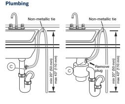
Note: Plumbing installations will vary - refer to local codes. Drain hose included is 88 5/8" (225 cm) and can be extended to a maximum of 165 3/8" (420 cm).
