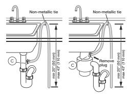
Note: Plumbing installations will vary - refer to local codes. Drain hose included is 88 5/8" (225 cm) and can be extended to a maximum of 165 3/8" (420 cm).
