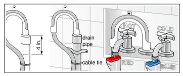
Attach the drain hose to the elbow included with your washer.
