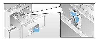
**NOTICE:** Do not use the liquid detergent insert with geltype detergents and powdered detergents or for cycles with pre-wash or selected "Finish in" time.
