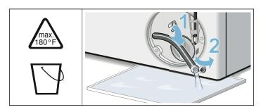
6. Turn the pump cover counterclockwise to remove it. A small amount of residual water may flow out when the cover is removed.
