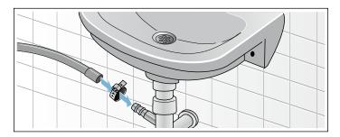
Secure the drain hose to the sink siphon using a Ø 0.9 - 1.6 in. (20-44 mm) hose clip (available from a hardware store).
