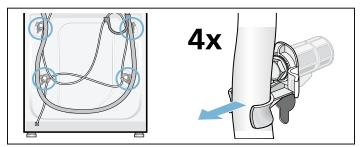
2. Loosen and remove all 4 transport bolts. Remove the sleeves. Take the power cable out of the brackets.
