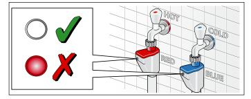
The AquaShield® hose prevents potential flooding in the event the hose develops an internal leak. If the hose leaks, the indicator turns red and water flow is blocked. Once the internal valve in the hose activates (indicator is red) the hose must be discarded. Contact customer service to purchase a replacement.
