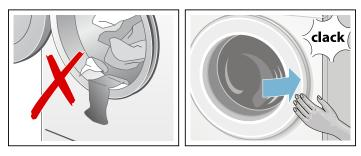
Foreign objects left in the drum may damage laundry. Before inserting any laundry, check to make sure no foreign objects are in the drum.
