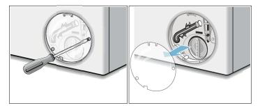
5. Use the pull-out drain hose located in the pump access opening to drain the remaining water into a suitable container (up to 5.3 U.S. gallons/20 liters of water may be drained). Pull the sealing cap from the hose and lay the hose over the side of the container and allow the water to finish draining from the drum. When finished, replace the sealing cap into the end of the hose and restore the hose to its storage location.
