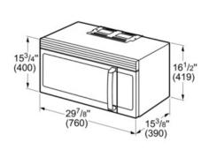
Measurements in inches (mm) in brackets
