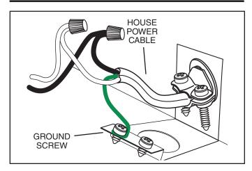
Connect <u>House Power Cable</u> to range hood wiring -BLACK to BLACK, WHITE to WHITE, and GREEN or BARE WIRE to <u>Ground Screw</u>. Replace electrical wiring box cover.
