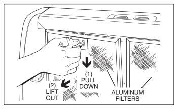
5 Remove the **Aluminum Filters** from the hood.
