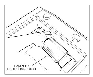
Remove 2 screws holding <u>Damper / Duct Connector</u> to hood. Remove damper/duct connector from inside the hood.
