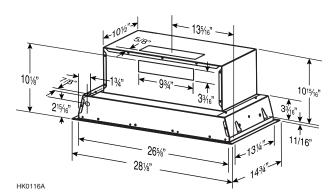
NOTE: The dual blower model has the same dimensions than the single blower model, but doesn't have an horizontal discharge. Refer to EC6230SSL illustration above for back and side dimensions, and discard horizontal discharge measurements.
