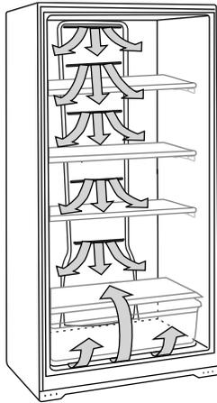
Do not block any of these vents with food packages. If the vents are blocked, airflow will be restricted, and temperature and moisture problems may occur.
