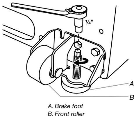
5. Make sure the freezer is steady. If the freezer seems unsteady or rolls forward when the door is pulled open, adjust the brake feet.
