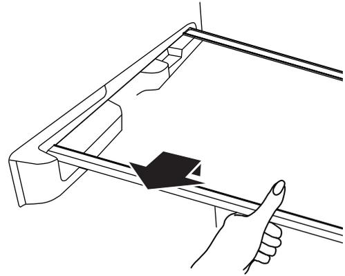
2. Replace the shelf by lowering the shelf onto the supports on the side wall.
