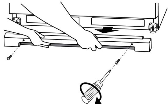
8. Replace the base grille by aligning the ends of the grille with the leveling assemblies on each side and snapping the grille into place. Reinstall the screws.
