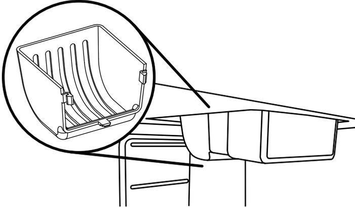
3. Replace bulb with a 40-watt maximum appliance bulb.
