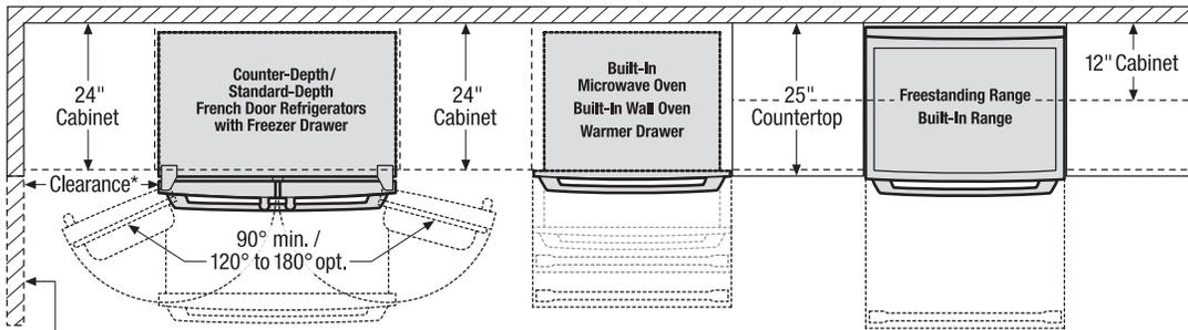
\*When installing a French door refrigerator adjacent to wall, cabinet or another appliance that extends beyond front edge of unit, 20" minimum clearance recommended to allow for optimum 120° to 180° door swing, providing complete drawer/crisper access and removal. (Absolute 4-1/2" minimum clearance will ONLY allow for 90° door swing which will provide limited drawer/crisper access with restricted removal.)
