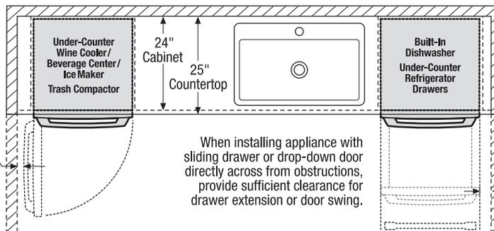
When installing appliance with side-swing door adjacent to wall, cabinet, or other obstruction that extends beyond front edge of appliance, door swing and handle clearance must be sufficient to allow access to appliance interior.
