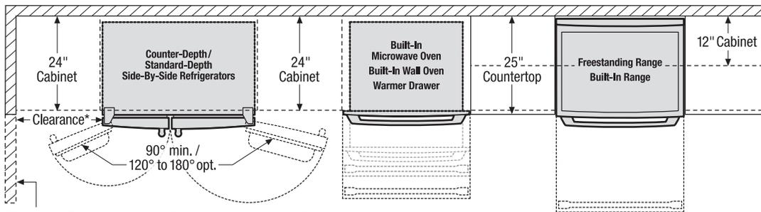
\*When installing side-by-side refrigerator adjacent to wall, cabinet or another appliance that extends beyond front edge of unit, 20" minimum clearance recommended to allow for optimum 120° to 180° door swing, providing complete drawer/crisper access and removal. (Absolute 4-1/2" minimum clearance will ONLY allow for 90° door swing which will provide limited drawer/crisper access with restricted removal.)
