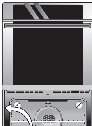
Double Wall Oven Serial Plate Location
