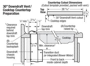
Maximum 41/2" gap allowed between inside cabinet back and chassis BEFORE downdraft stabilizing brackets will require wood support installation for mounting
