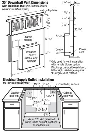
Electrical Installation Notes: All vertical dimensions relative to top surface of countertop; all horizontal dimensions relative to cutout in countertop. Locate grounded electrical outlet for 28"-long power cord within reachable distance. When installing vent in 30"-wide cabinet, outlet cannot be located on back wall of cabinet, but can be wall-mounted with access hole in cabinet. Ensure that access to outlet will NOT be obstructed by ducting after installation.
