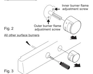
Test to verify if "LO or LOW" setting should be adjusted (right front position ONLY):
