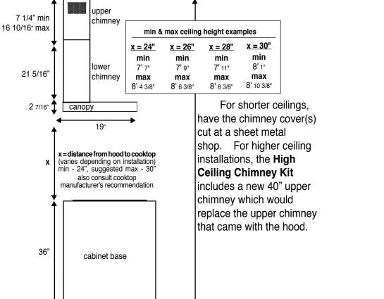
Make your ductrun as straight and short as possible. The ductrun should not exceed 35 equivalent feet if ducted with the required minimum of 6" round duct. Count 45° angles as 3 feet, 90° elbows as 5 feet, and 90° flat elbows as 12 feet.
