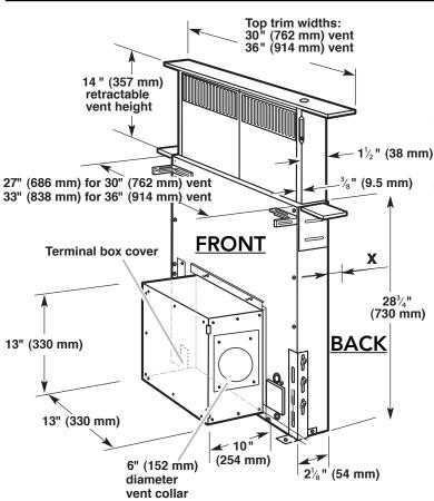
Note: Overall dimensions show unit with internal blower box attached. Remote
