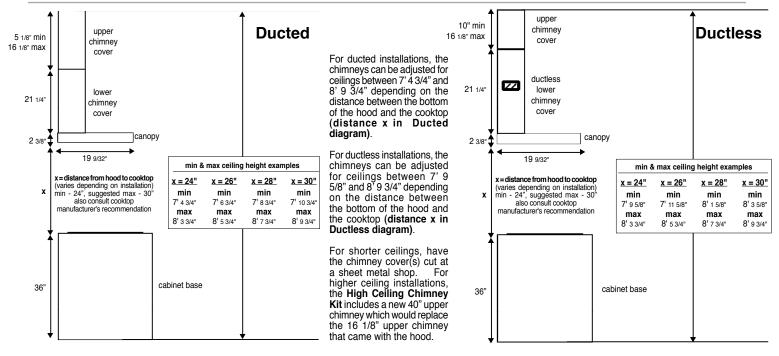
Note: If 24" or 30" High Backsplash is being installed, the distance between the bottom of the hood and the cooktop (distance x in diagram) is equal to the height of the Backsplash.
