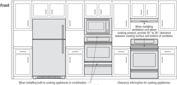
2"-high minimum visible gap between appliance faceplates required.
