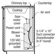
\*Blower can be adjusted to allow for accurate alignment of ductwork to floor joists, wall studs, electrical wiring or plumbing
