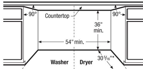
**Side-by-Side Units in Under-Counter Installation**
