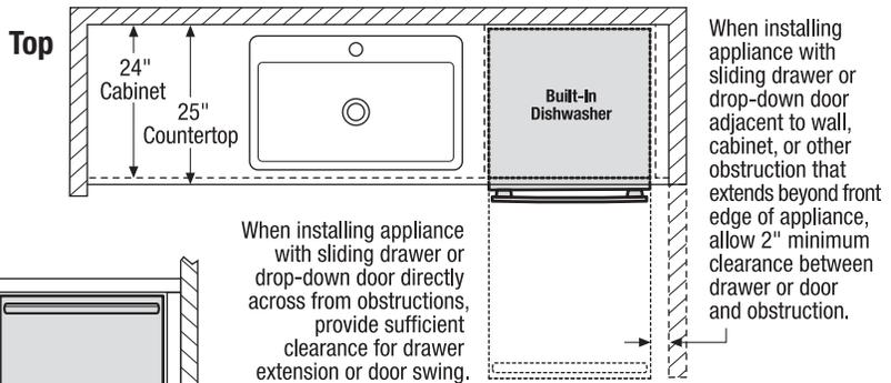
When installing appliance with sliding drawer or drop-down door directly across from obstructions, provide sufficient clearance for drawer extension or door swing.
