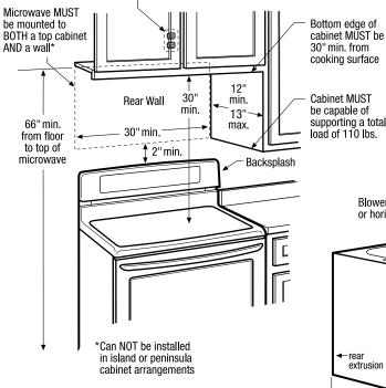
Locate 120V/60Hz grounded outlet inside upper cabinet
