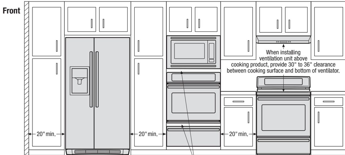
When installing appliances adjacent to each other, 20" minimum distance between each appliance required.
