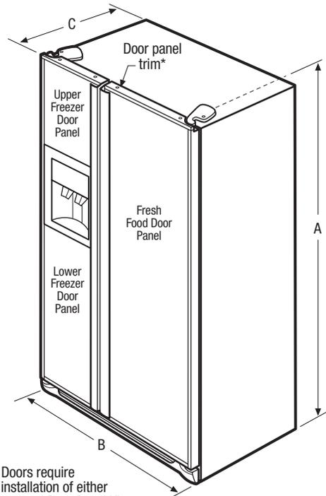
\*Doors require installation of either optional Door Panel Kit or custom-built door panels.
