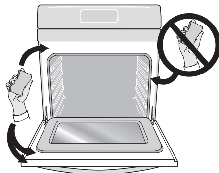
Figure 6: Clean around the oven door gasket
