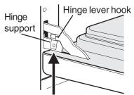
Lock engaged for door removal Figure 1
