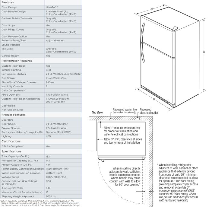
For use on adequately wired 120V, dedicated circuit having 2-wire service with a separate ground wire. Appliance must be grounded for safe operation
