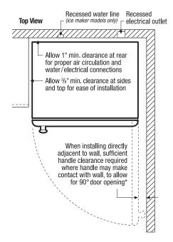
\* When installing refrigerator adjacent to wall, cabinet or other appliance that extends beyond front edge of unit, 20" minimum clearance recommended to allow for optimum 140° door swing, providing complete crisper access and removal. (Absolute 3" minimum clearance will ONLY allow for 90° door swing which will provide limited crisper access with restricted removal.)
