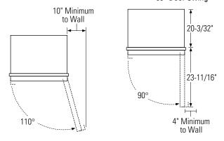
• The door swing is reversible on all models. If desired, change the door swing before installation.
