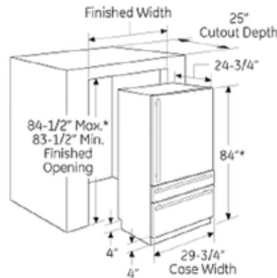
\*84" high installation. The wine reserve can be adjusted to fit into a cutout that is 83-1/2" min. to 84-1/2" max. with the appropriate door kit. Use leveling legs and wheels for a maximum 1" height adjustment.
