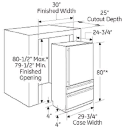
\*80" high installation. The wine reserve can be adjusted to fit into a cutout that is 79-1/2" min. to 80-1/2" max. height. Use leveling legs and wheels for a maximum 1" height adjustment.
