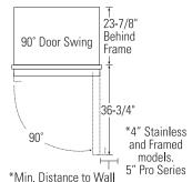
Allow 25" minimum clearance for a full 130° door swing. Allow 15" for pan removal.
