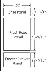
IMPORTANT NOTE: Maximum total weight for the assembled panels: Door panel – 67 lbs. Grille Panel – 18 lbs.
