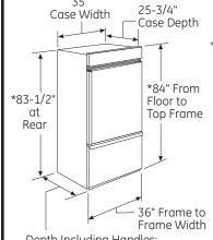
\* Shipping height. The refrigerator can be adjusted to fit into a cutout that is 84-1/2" max. height. Note that the top case trim at the front is 1/2" higher and will overlap upper cabinetry or soffit. Use leveling legs and wheels for a maximum 1" height adjustment.
