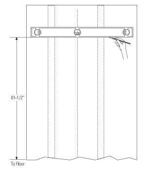
Locate at least 2 studs on the back wall. Mark these points on the horizontal line.
