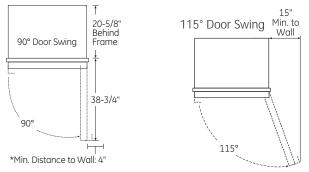
For a 90 degree door swing, allow 4" min. clearance to wall. If the 90 degree door stop position is used, pan access is maintained, but pan removal is restricted
