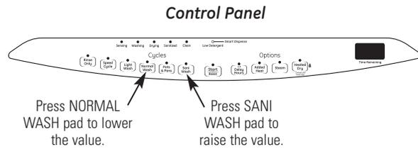
3. Press the **SANI WASH** pad to raise the value or the **NORMAL WASH** pad to lower the value. Set the water hardness value (**1 to 5**) to the number determined with the test strip and table at left.
