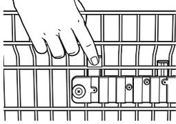
The upper rack is adjustable (on some models) to add flexibility in loading your dishwasher. To lower, push tabs in and lower rack. To raise, just pull up on rack until it snaps.
