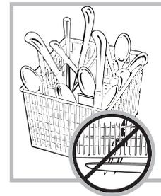
**Do not let any item extend through the bottom of the silverware basket. Items that extend through the rack could prevent the spray arm from turning and cause poor wash performance.**
