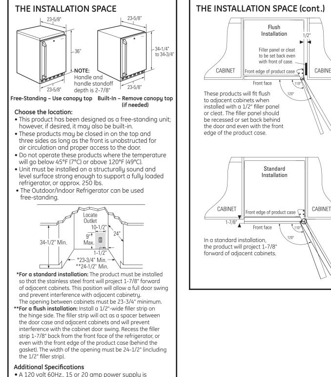
required. An individual properly grounded branch circuit or circuit breaker is recommended. Install a properly arounded 3-prong electrical receptacle recessed into the back wall as shown. Electrical must be located on rear wall as shown. THIS PRODUCT MUST BE CONNECTED TO A POWER SOURCE WITH GROUND FAULT CIRCUIT INTERRUPTER (GFCI) PROTECTION WHEN INSTALLED IN AN OUTDOOR LOCATION. LOCAL CODES MAY REQUIRE A SEPARATE CIRCUIT.
