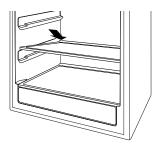
Place in slots when replacing the shelf
