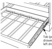
Tab (push tab down on right drawer guide, pull tab up on left drawer guide)
