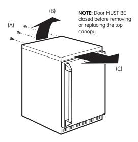
**CAUTION:** Under side edges of the stainless steel canopy top may be sharp. Wear heavy-duty work gloves when moving the top.
