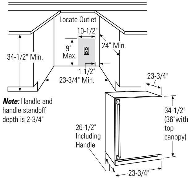
**Note:** If installing between frameless cabinets, a 1/2" wide filler strip or side panel may be required. The filler strip will act as a spacer between the door case and adjacent cabinet and will prevent interference with cabinet door swing. The width of the opening must include filler panels.
