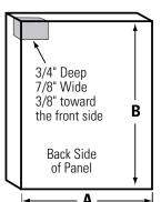
3/4" Overlay Panel Dimensions (in inches) A (Width) B (Height) 23-3/16" 29-9/16" 1/4" Backer 0.10" Spacer 22-1/2" 29-1/16" 3/4" Overlay 23-5/8" 30' NOTE: Max. assembled drawer panel weight
