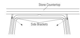
• Fasten the brackets to the cabinet sides using the 2 Phillips head wood mounting screws. IMPORTANT: Drive screws straight and flush. Protruding screw heads may scratch the top or sides of the control panel and can interfere with door closing.
