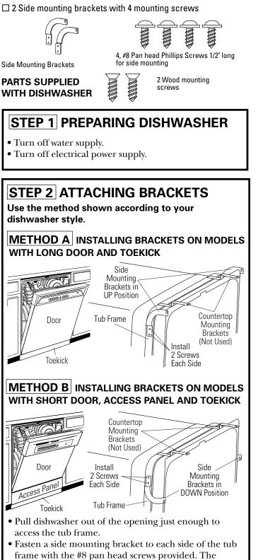
bracket should be installed, as shown for your model.
