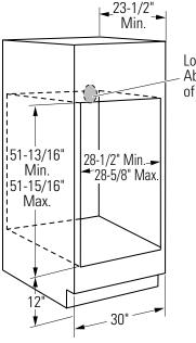
Locate Junction Box 47" Above Cutout Floor, Within 5" of Right Rear Wall
