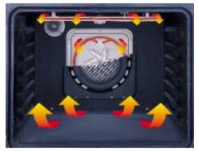
Spectra ranges deliver "true European convection" cooking by means of a third dual-loop heating element located in the back wall. A fan evenly circulates air throughout the oven cavity. This process delivers uniform, savory results.
