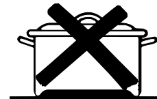
Pans with rounded, curved, ridged or warped bottoms are not recommended. Pan detection/sizing may not work properly with these types of pans.
